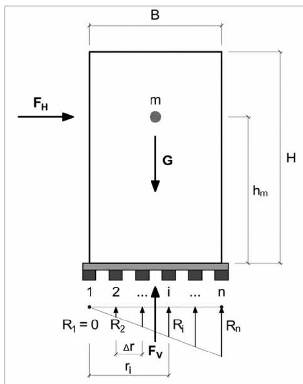
Figure 4: External forces and base reactions of a base isolated rigid body just before entering the rocking phase.
